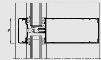
Concept Wall® 50 is a façade and roof system that offers unlimited design freedom and allows maximum transparency. As such, CW 50 meets all requirements of contemporary architecture. Innovative solutions contribute towards the tendency of big, heavy and thick glass panes. CW 50 supports up to 150, 310 and even 600 kg in various glass support configurations.
